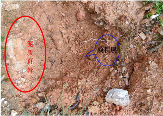
图2 松软的残积层特征 Fig.2 Features of soft residual strata
