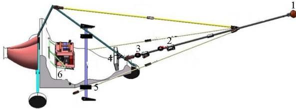
1—铯光泵磁探头;2—磁通门三分量传感器;3—实时差分 GPS 天线;4—导航显示屏;5—高度计;6—数据采集器、补偿器 1—cesium optical pump magnetic probe;2—fluxgate three component sensor;3—real time differential GPS antenna;4—navigation display;5—altimeter;6—data collector, compensator
