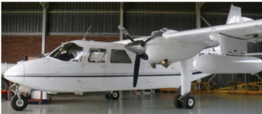
图 2 安装航空重(磁、放)的 BN-2T 飞机 Fig.2 BN-2T aircraft installed with airborne gravity, magnetic, radiation
